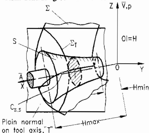
Fig.8 - "Plain Generating Curves" method applied to profile an end-mill cutter
