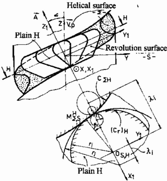
Fig. 4 The "substituting circles family" method. Contact between a helical and a revolution surface
